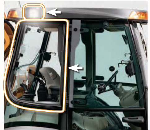
New rear-quarter windows and side lighting
