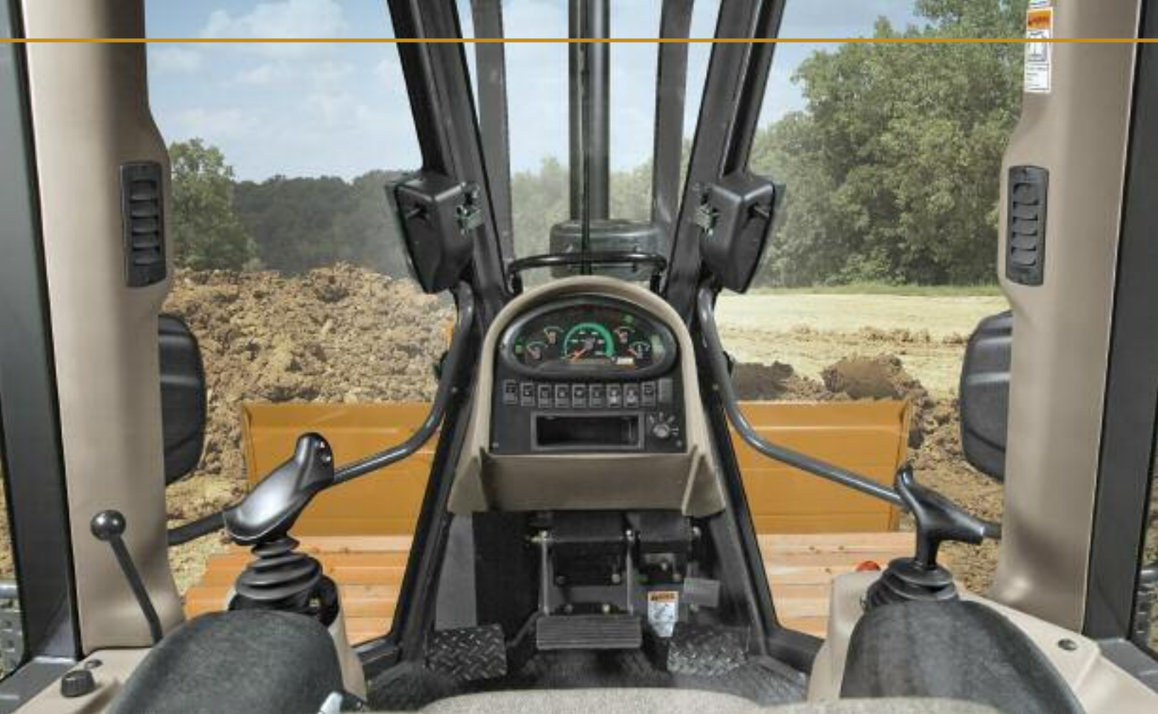
The L Series cab features a large glass area that provides an excellent view to the blade and work area.
