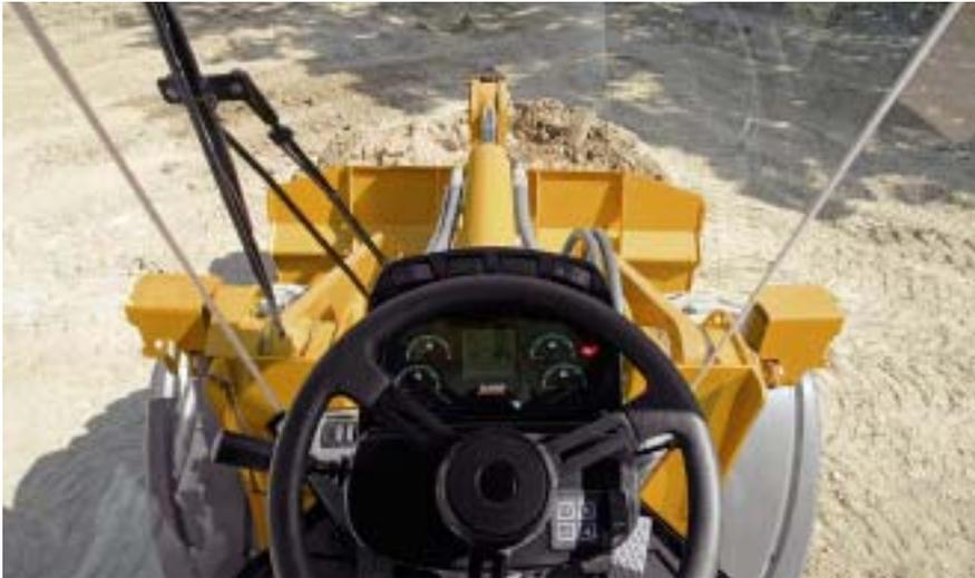
An unobstructed view to the console's analog gauges and indicator lights keeps you informed of critical machine functions.
