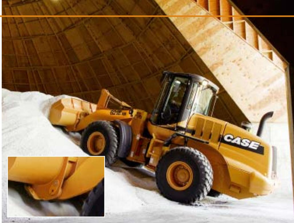
E Series buckets feature an extended bolt-on cutting edge for easier penetration into the pile. The hinge pins are raised up out of the dirt and debris for longer life.
