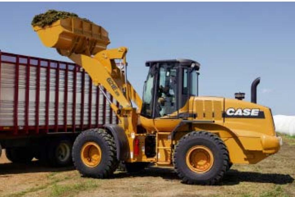
The XR configuration supplies all the benefits of the Z-bar configuration but with an added advantage of extended reach.
